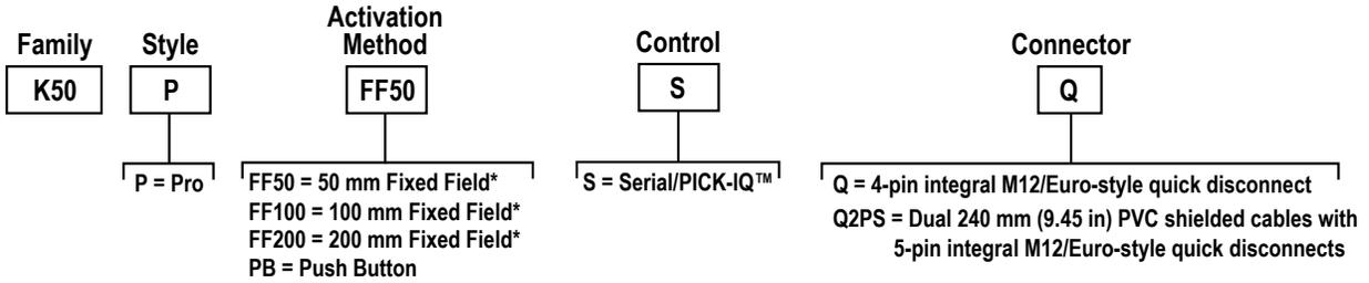
\*Cutoff distance will vary from specified range based on target and tolerances
