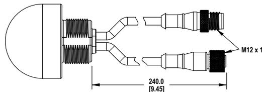
**Note:** The splitter cordset dimensions are functionally identical for all K50 devices; the K50 Indicator is shown.
