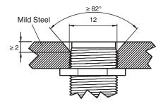
Sensor face is flush with mounting surface.
