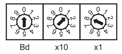
Internally, 1 is always added to the node number to avoid setting of the node number 0.
