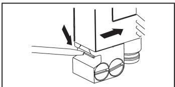
▶ To remove the unit press the spring down with a screwdriver and slide the unit out.
