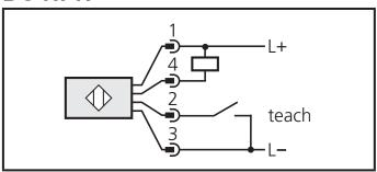
Programming of the output function by pushbutton or programming wire ( $\rightarrow$  6.4 Programming the output function).
