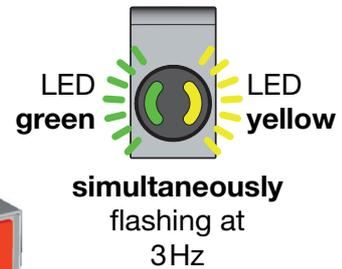
**Teach for increased sensor sensitivity (highly transparent bottles and foils with thickness < 20µm)**
