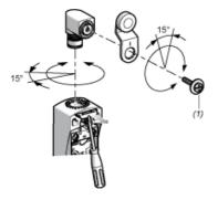
(1) Tightening torque (Min: 1) (Max: 1.5)
