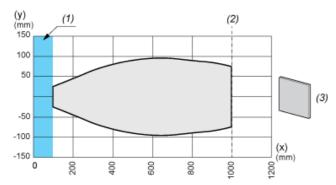
(X): Target distance (Y): Detection limit
