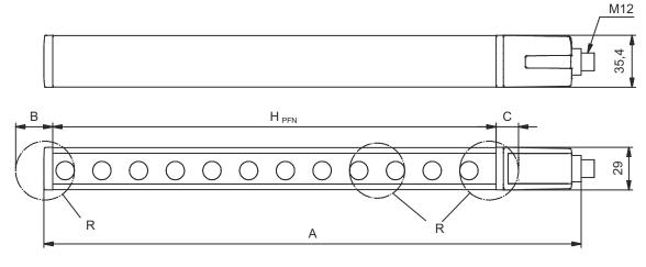
$H_{\mathrm{PFE}}$  Effective protective field height = 467 mm  $H_{\mathrm{PFN}}$  Nominal protective field height = 450 mm
