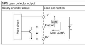
XBe sure that if overload or short-circuit to output terminal, output circuit is damaged.
