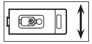
The objects to be detected are to move tranversally to the lens of the unit. In case of other directions of movement it should be tested before whether safe functioning is guaranteed.
