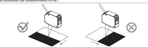
Step surface or segment gap measurement(Install in the direction shown in the figure below to reduce impact by step edges in measurement)
