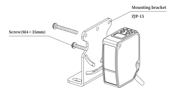
\*For mounting, please keep tightening torque < 0.5N·m
