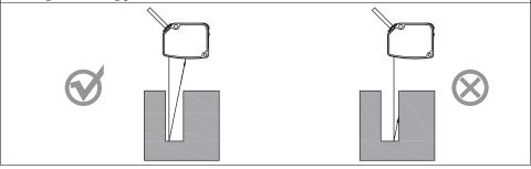
Measurement for wall surface mounting(Install in the direction shown in the figure below to reduce the multiple reflected light from the wall surface, since the reflected light will enter the receiving surface. In case of wall surface high reflection rate, it is better to change to matte black)
