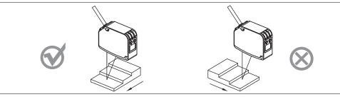
Measurement of rotating objects(Mounting in the direction shown in the figure below to control impact by vertical vibration and position deviation of the object)
