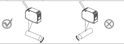
Measurement in narrow places and recessed parts(For installation and measurement in narrow places and holes,take care to avoid blocking the light path from the light-emitting part to the light-receiving part)
