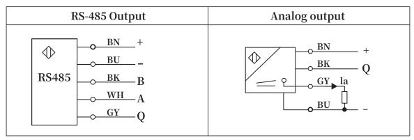
Remark: The sensors are equipped with shielded cables,Q is the switch output.
