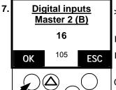
Indicates that the fieldbus module 11 (digital input master 2B) with a length of 16 bytes is activated.
