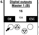
Indicates that the fieldbus module 6 (digital output master 1B) with a length of 16 bytes is activated.
