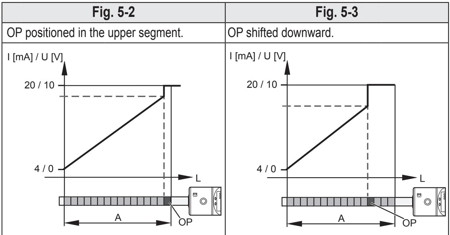
A: Active zone      OP: Measuring segment overflow prevention OP      L: Level
