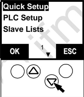
Press [▼] to scroll to [PLC Setup]
