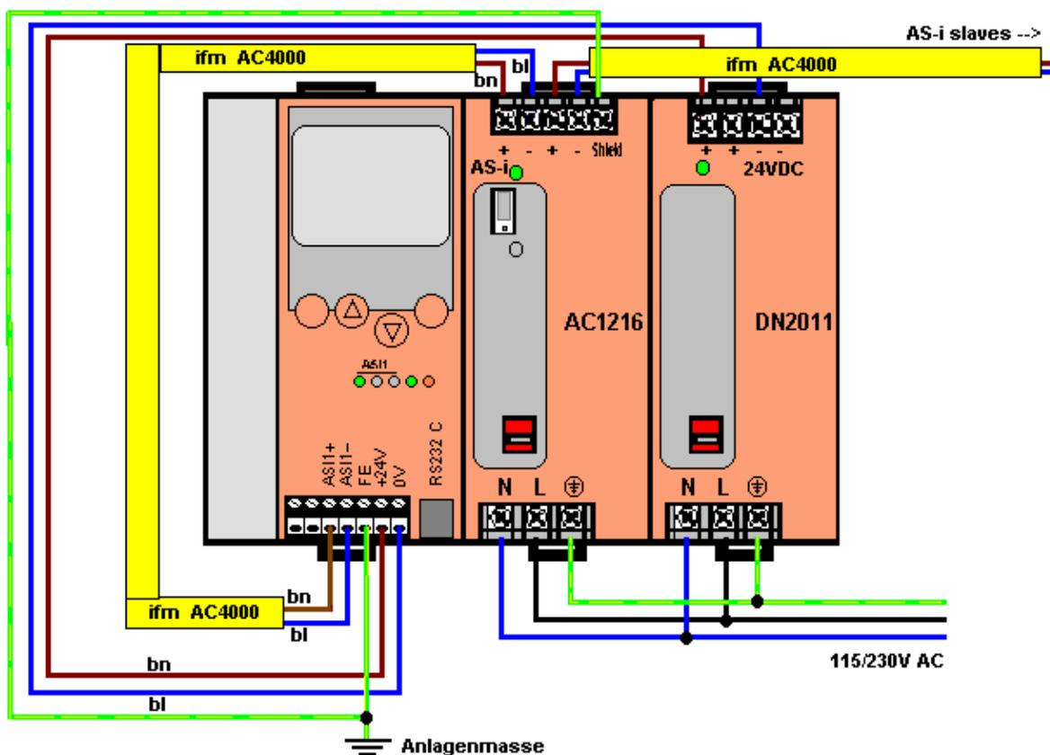
Figure: suggestion for wiring the controller
