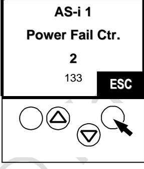
> Display of the number of failures of the AS-i supply on the master
