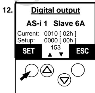
▶ Transmit the setup value set with [SET] to the outputs of the slave
