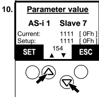
> Display of current and setup parameter values as binary value and hex value
