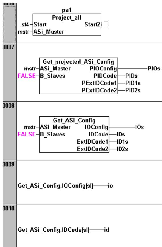
Function block: All slaves detected on master "mstr" are entered as projected in the LPS of the controller.
