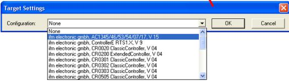
▶ Select a valid target for the controller and confirm with [OK]
