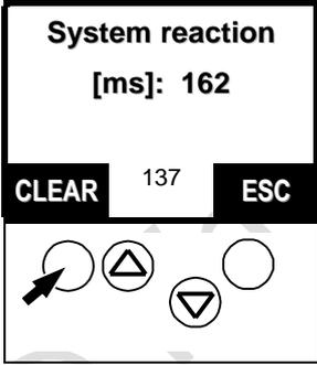
> Display of the longest cycle time of the AS-i system in [ms] since the last reset
