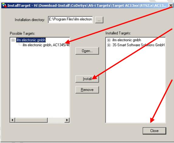
▶ Mark the target for the controllere (→ figure)
