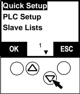
Press [▼] to scroll to [PLC Setup]
