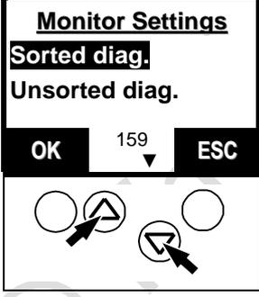
> Display of the current setting of the safety monitor (marked line = active):
