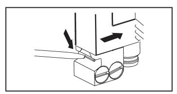
▶ To remove the unit press the spring down with a screwdriver and slide the unit out.
