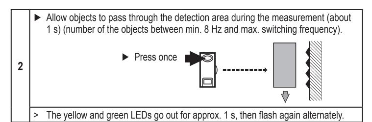
► Allow objects to pass through the detection area during the measurement (about 1 s) (number of the objects between min. 8Hz and max. switching frequency).
