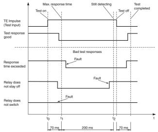
The door controller must query the sensor at times t<sub>1</sub> and t<sub>2</sub>.
