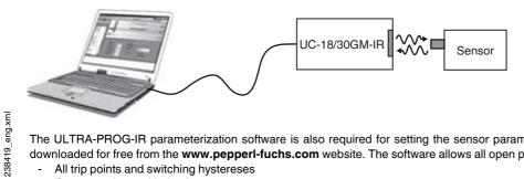
The ULTRA-PROG-IR parameterization software is also required for setting the sensor parameters. The ULTRA-PROG-IR software can be downloaded for free from the www.pepperl-fuchs.com website. The software allows all open parameters to be set, including:
