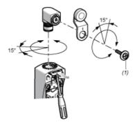
(1) Tightening torque (Min: 1) (Max: 1.5)
