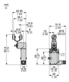
(1) 2 fixing holes  $\emptyset$  4.2 mm, counterbored  $\emptyset$  8 mm by 4 mm deep.
