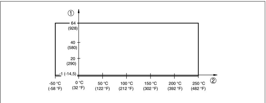
Fig. 27: Process temperature - Process pressure with switch position 0.7 g/cm<sup>3</sup> (mode switch)
