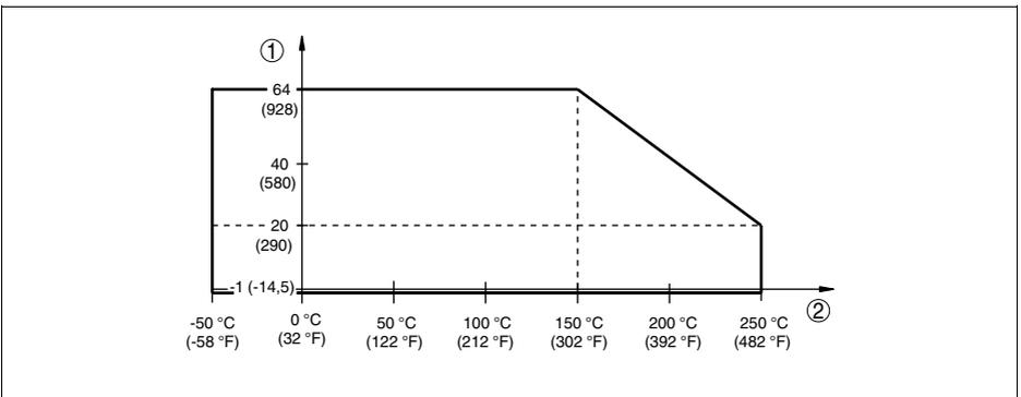
Fig. 28: Process temperature - Process pressure with switch position 0.5 g/cm<sup>3</sup> (mode switch)
