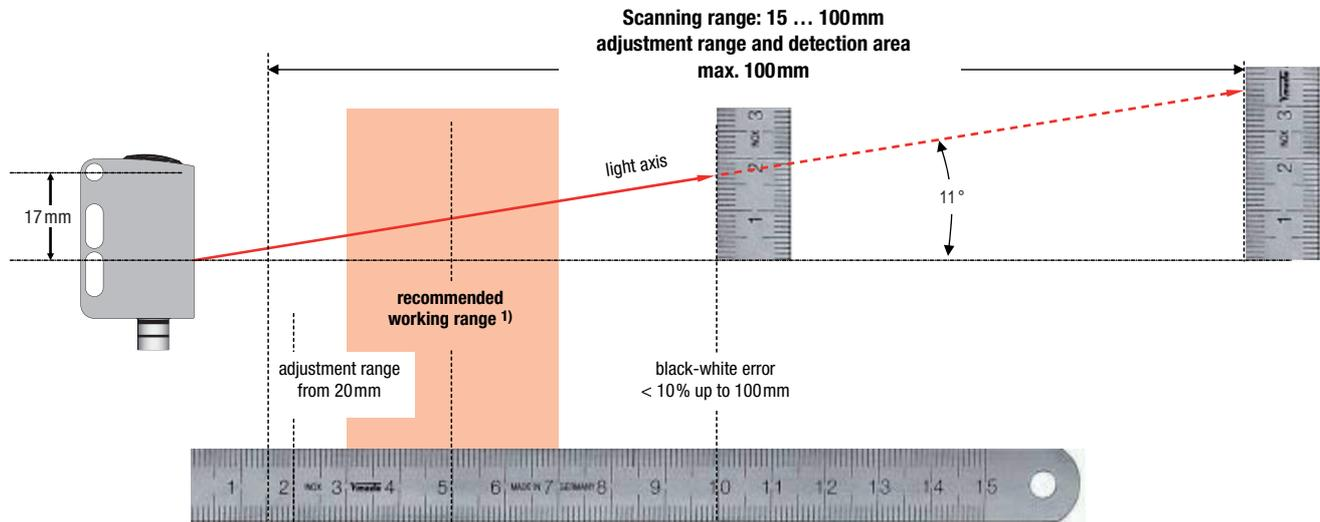
1) The sensor is most capable of reliably detecting a reflective surface or transparent object in the recommended working range. Nevertheless, the sensor can reliably detect such objects in the entire scanning range; however, the performance reserve is reduced as compared with the recommended working range.
