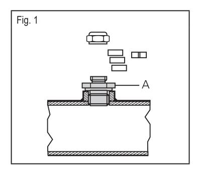
► Insert the fitting (A) into the process connection and tighten it.
