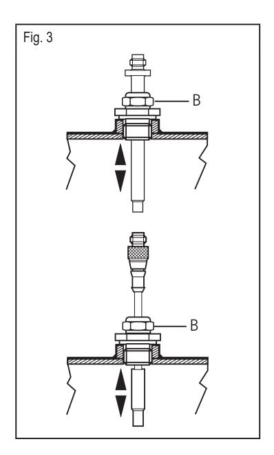
➤ Adjust the sensor to the required installation depth and tighten the coupling nut (B).
