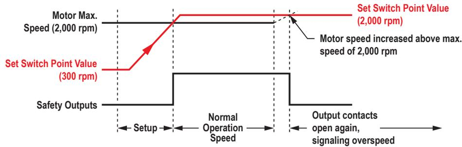
Figure 9. Over-speed Timing
