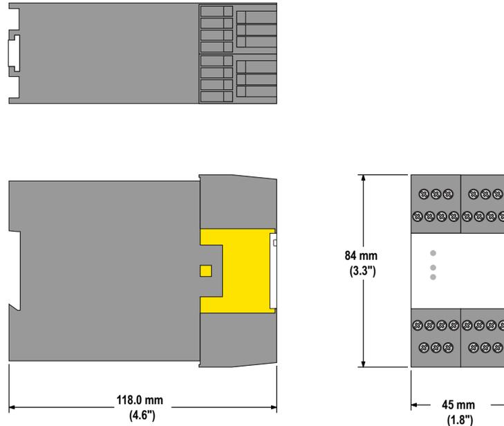
Figure 10. Dimensions—SSM-FM-11A20
