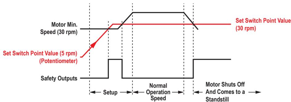
Figure 8. Under-speed Timing
