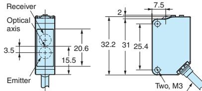
4-dia. vinyl-insulated round cable with 3 conductors (Conductor cross section: 0.2 mm<sup>2</sup>, Insulator diameter: 1.1 mm), Standard length: 2m
