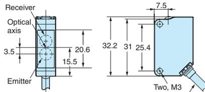
4-dia. vinyl-insulated round cable with 4 conductors (Conductor cross section: 0.2 mm<sup>2</sup>, Insulator diameter: 1.1 mm), Standard length: 2m
