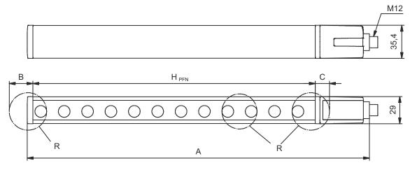
$H_{\mathrm{PFE}}$  Effective protective field height = 540 mm  $H_{\mathrm{PFN}}$  Nominal protective field height = 450 mm
