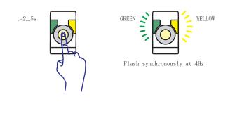
Note: For distancing setting, if the distance between the sensing object and the sensor exceeds the detection ability of the product, in duration  $2s \leq t < 5s$ , the yellow and green lights flash synchronously at 4Hz, when the button is released to finish the distance setting but not successfully.
