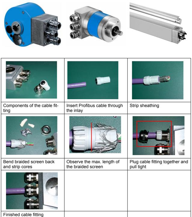
Figure 10–1: Screen Connection at the Bus Link Adapter with Cable ATM60-P/ATM90-P/ KHK53-P.
