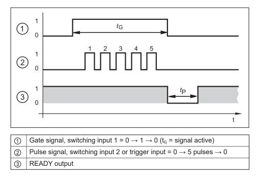
While there is an active signal on switching input 1 (gate signal), the device counts incoming pulses and activates the respective application.
