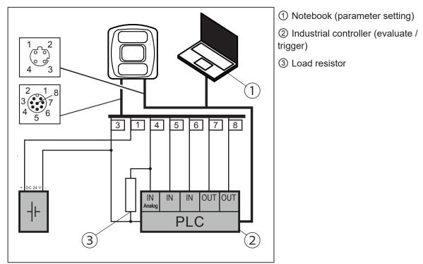
Using the ifm Vision Assistant software it is possible to assign one process value each to the start value (4 mA / 0 V) and the end value (20 mA / 10 V) of the analogue output.
