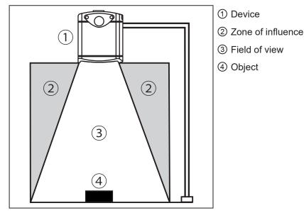
Optimum detection of an object ④ is given if the following conditions are met:
