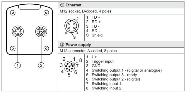
Cover unused Ethernet connection with the protective cap (E73004). Tightening torque 0.6...0.8 Nm.
