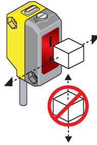
Figure 2. Optimal Orientation of Target to Sensor
