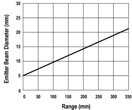
Figure 6. Typical Emitter Spot Diameter vs. Distance
