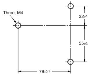
Mounting Hole Dimensions for Operation Key
