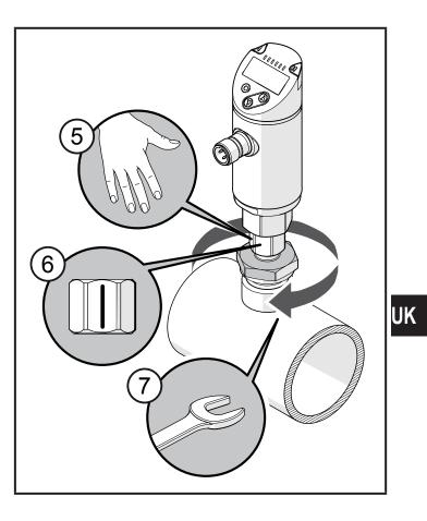
> The cutting ring is now firmly connected to the sensor probe. The installation depth can no longer be changed.
