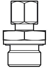
The progressive ring fitting consists of the four parts screw fitting (1), first clamping ring (2), second clamping ring (3) and coupling nut (4).
