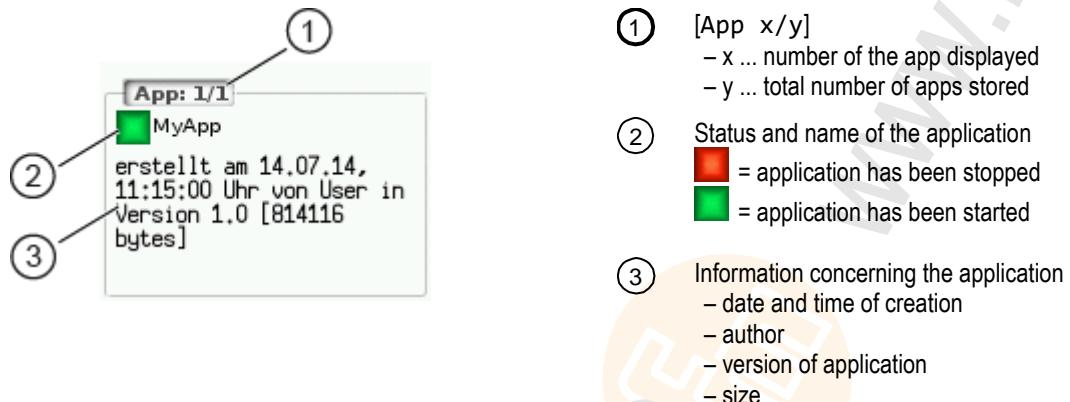
To control a single PLC application stored on the device:
