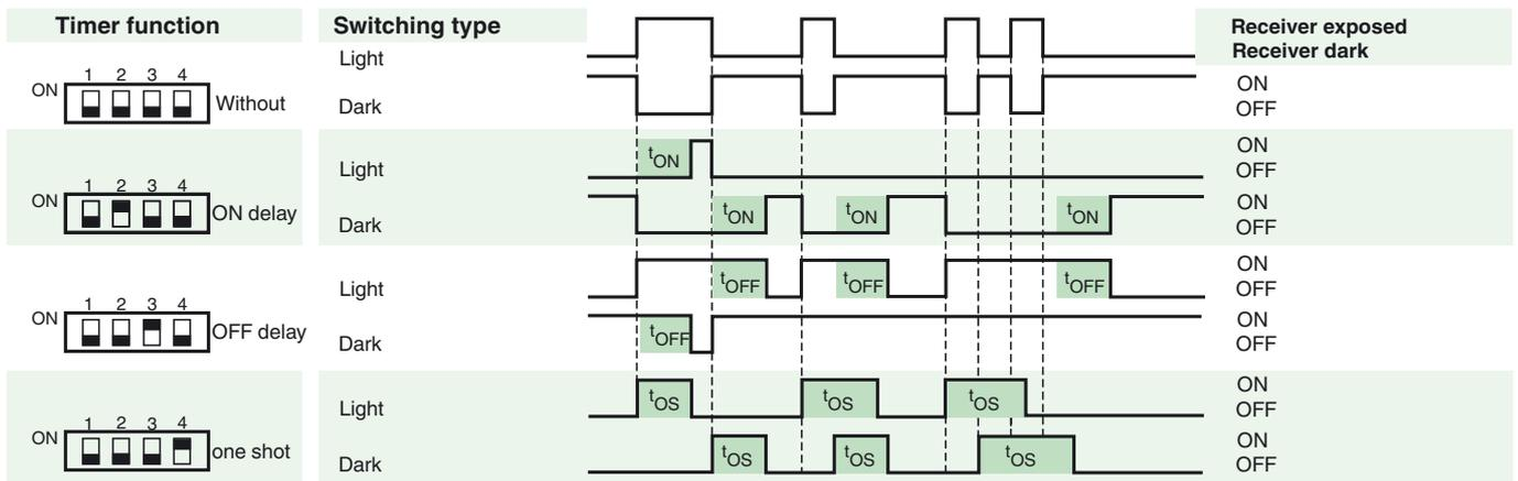
Time  $t_{ON}$ ,  $t_{OFF}$  and  $t_{OS}$  are adjustable from 0.02 to 1 seconds.
