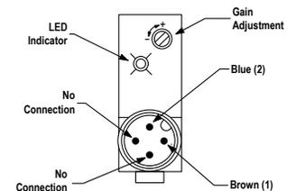
Figure 1. Features (rear of sensor, quick-disconnect model shown)
