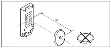
► Align the ID tag on the antenna central axis
