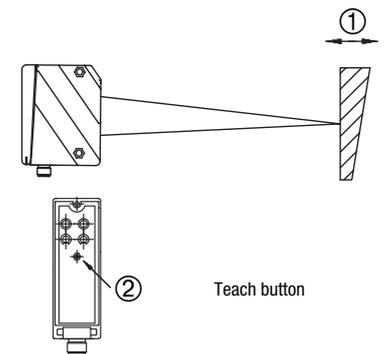
3. Release teach button (②) and wait for optical confirmation by end of flashing signal (green LED on).
