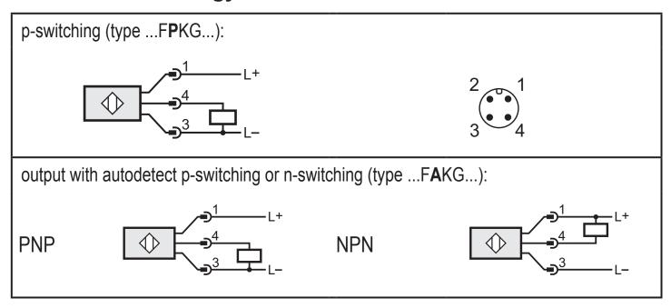
On power up, the unit detects automatically if the output is connected to L- (= PNP) or to L+ (= NPN).
