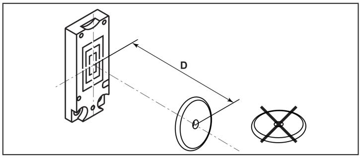
► Align the ID tag on the antenna central axis
