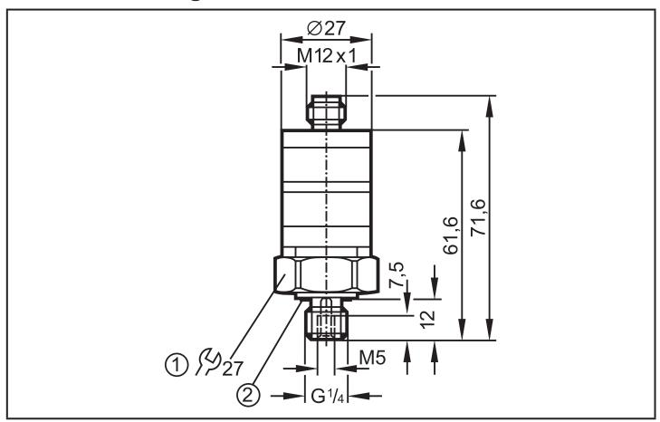
Dimensions are in millimeters (25.4 mm = 1 inch)
