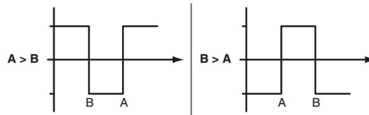
Teach in switching thresholds: you can teach in or overwrite a taught-in switching threshold at any time. To do this, press the "TI" button again.
