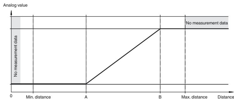
**Falling slope (A > B)**
