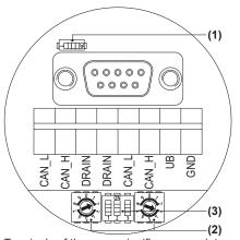
Terminals of the same significance are internally connected and identical in their functions. Max. load on the internal terminal connections UB-UB and GND-GND is 1 A each.
