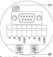
Terminals of the same significance are internally connected and identical in their functions. Max. load on the internal terminal connections UB-UB and GND-GND is 1 A each.
