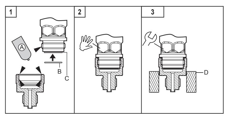
Slightly grease the threads and sealing areas of the sensor and adapter with the lubricating paste (A).
