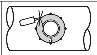
Apply the welding seams between the fixing points opposite each other. Ensure sufficient intervals between the individual sections to avoid glowing through or warping of the adapter due to overheating.
