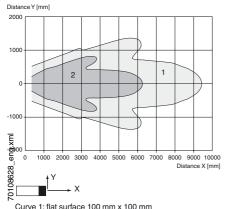
Curve 1: flat surface 100 mm 82 Curve 2: round bar, Ø 25 mm 000 cience 2: round bar, Ø 25 mm
