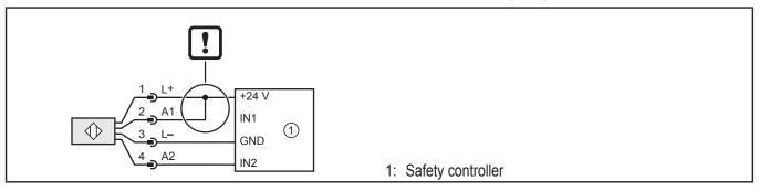
► Connect A1 to the sensor's positive supply.
