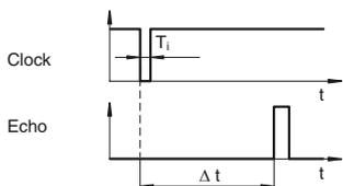
We recommend the usage of a npn-transistor to trigger the sensors clock input. The sensors clock input is connected to the  $+U_B$  potential internally by means of a pull up resistor.
