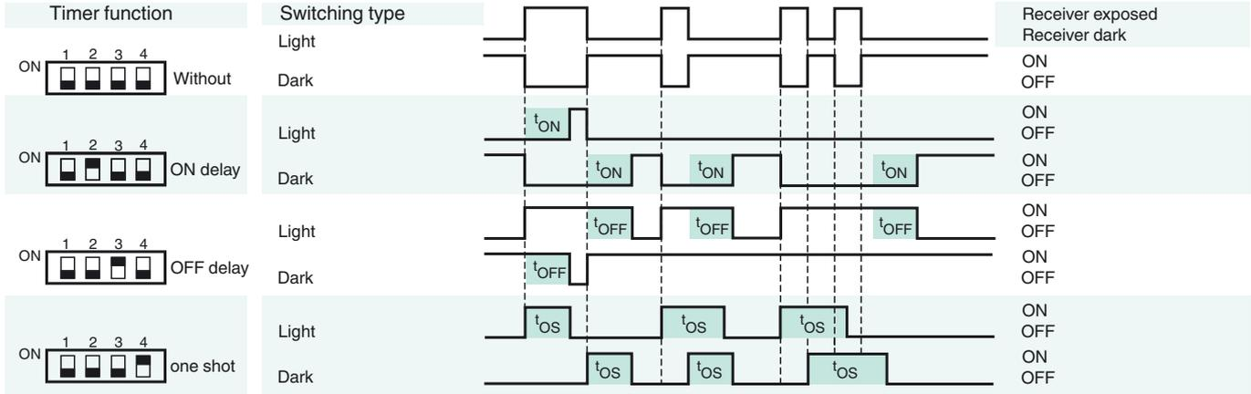
Time  $t_{ON}$ ,  $t_{OFF}$  and  $t_{OS}$  are adjustable from 0.1 to 10 seconds.
