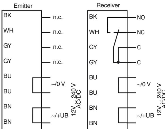
The relay-functions "NC" and "NO" bear on the switching mode "Dark-ON". This complies to the default setting of the light/dark switch (factory setting).
