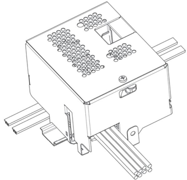
▶ Attach the cover, clip it into place and tighten the screw
