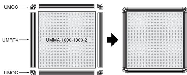
In this case, the perimeter of the Safety Mat is about 4 m and the following pieces are required:
