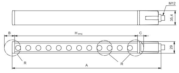
$H_{\mathrm{PFE}}$  Effective protective field height = 3040 mm  ${\rm H}_{\rm PFN}$  Nominal protective field height = 3000 mm
