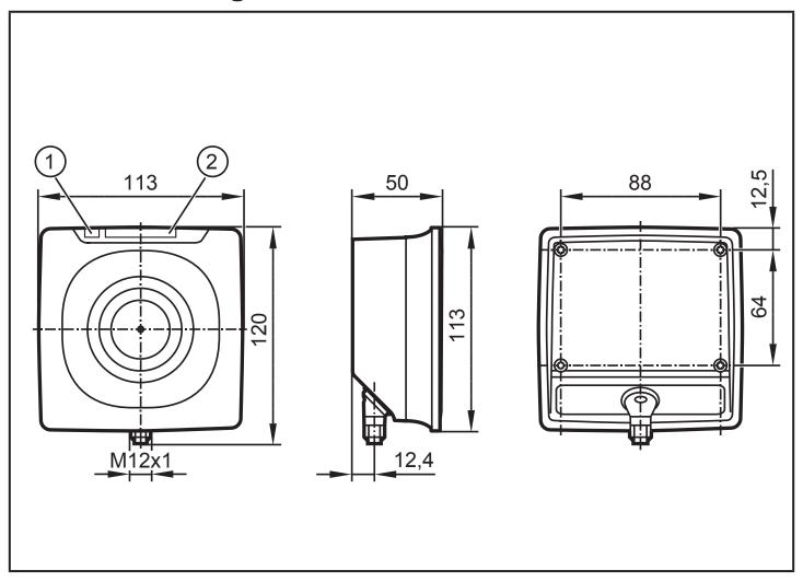
The max. tightening torque of the screws when mounting the unit is 0.8 Nm.
