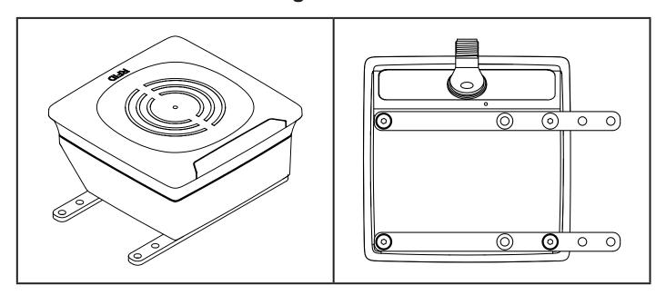
► Fix the unit with fixing screws to the designated location.
